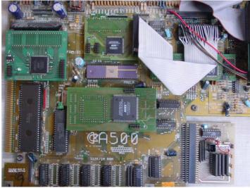
Clone-A development chips mounted on adaptor boards in place of the custom chips of an A500 motherboard. By developing this way, the Clone-A chipset will be extremely close to the original Amiga chipset.
