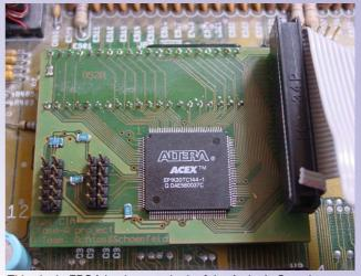
This single FPGA implements both of the Amiga's Complex Interface Adaptor (CIA) chips.
