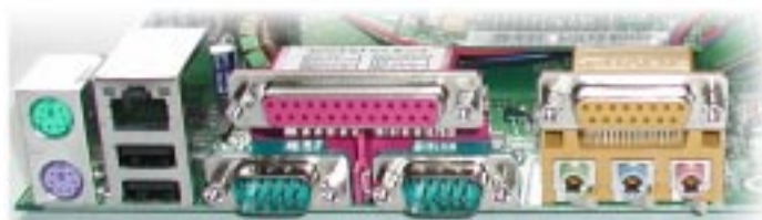
AmigaOne-XE connectors, from left to right: PS/2 keyboard and mouse, USB & Ethernet, parallel & serial, game port, audio I/O.
